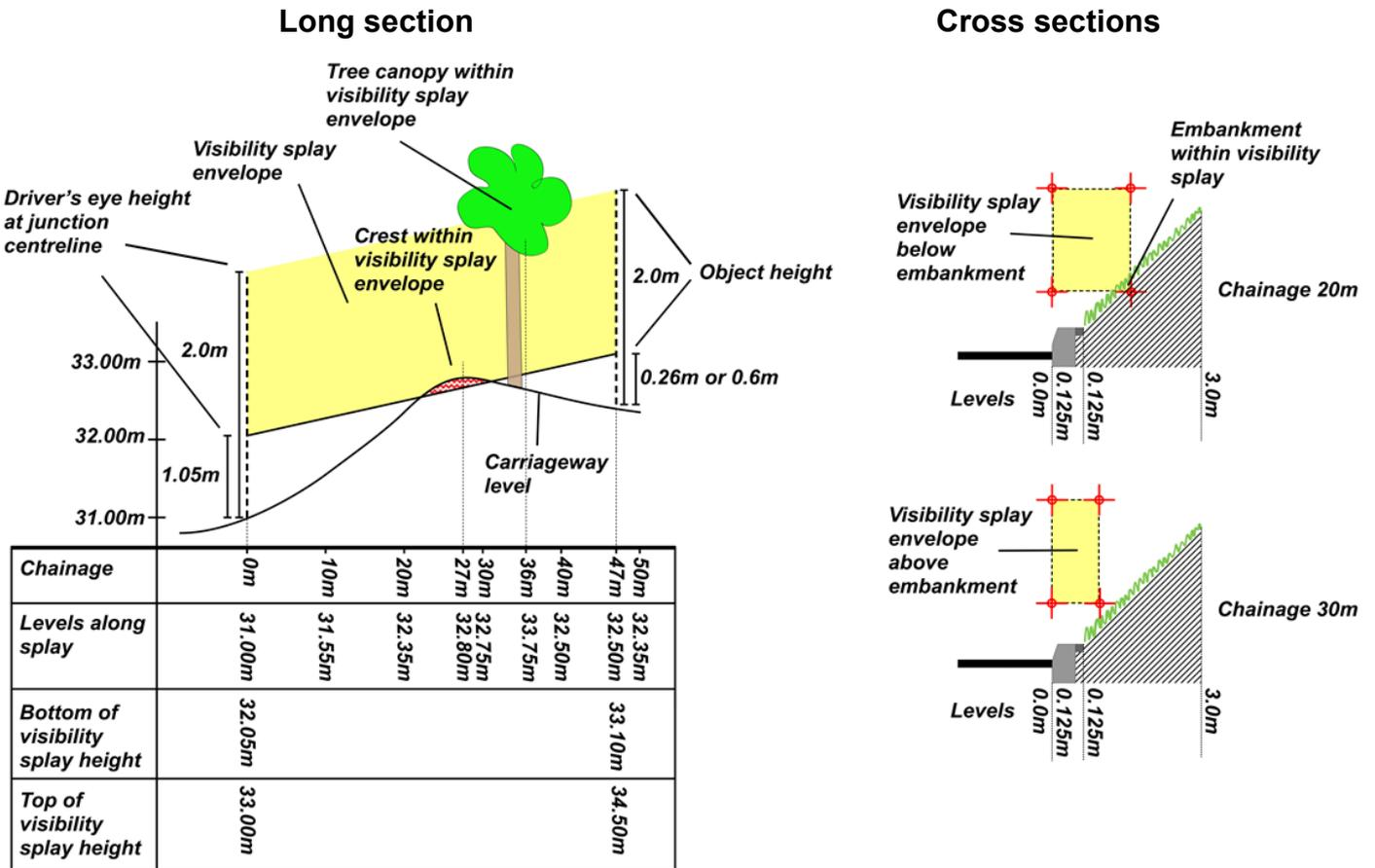
3.3.14 It is accepted that a visibility splay may be more accurately plotted by measuring the Y-distance along the inside wheel track. The likely position of the wheel track from the edge of the carriageway will vary depending on the width of the carriageway and roadside features. This must not be overestimated.
