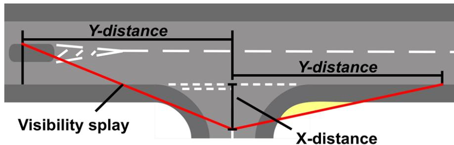
3.3.7 Where there is a wide splitter island within the mouth of the junction or more than one junction approach lane, it will be more appropriate to measure the X-distance from the actual position of the driver. The measurement of the Y-distance is then adjusted accordingly.
