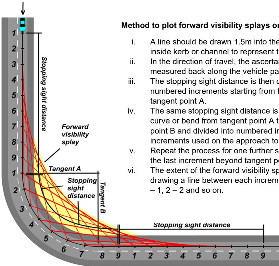
**Method to plot forward visibility splays on curves and bends**
