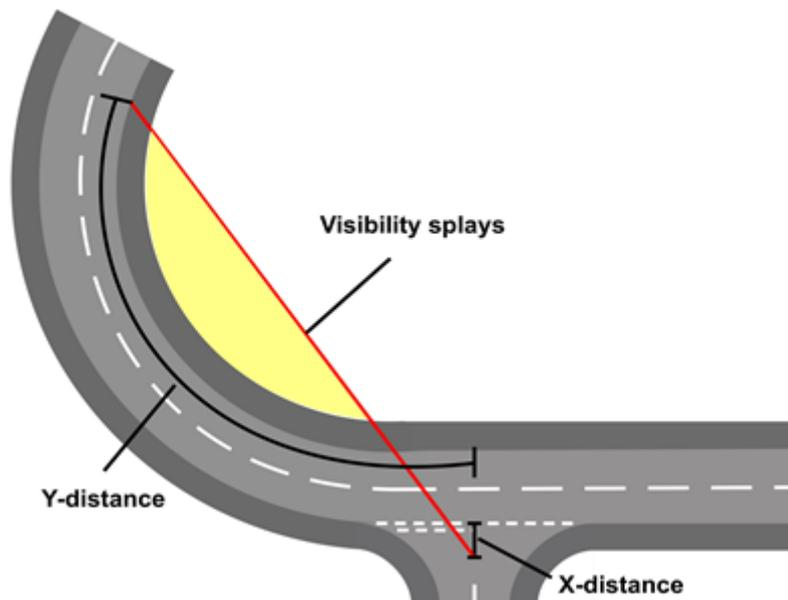
**Notes:** Visibility splays must be either within the public highway or over land in the control of the developer to ensure that they remain free from obstruction whilst ever the development remains in existence. Hedges should not be planted within 1.0m of the visibility splay if there is potential for the visibility splay to be encroached upon by vegetation during periods of rapid growth.
