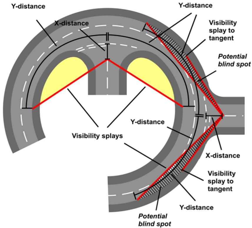
**Priority junction and direct access offside visibility splays when emerging on to a curved street**
