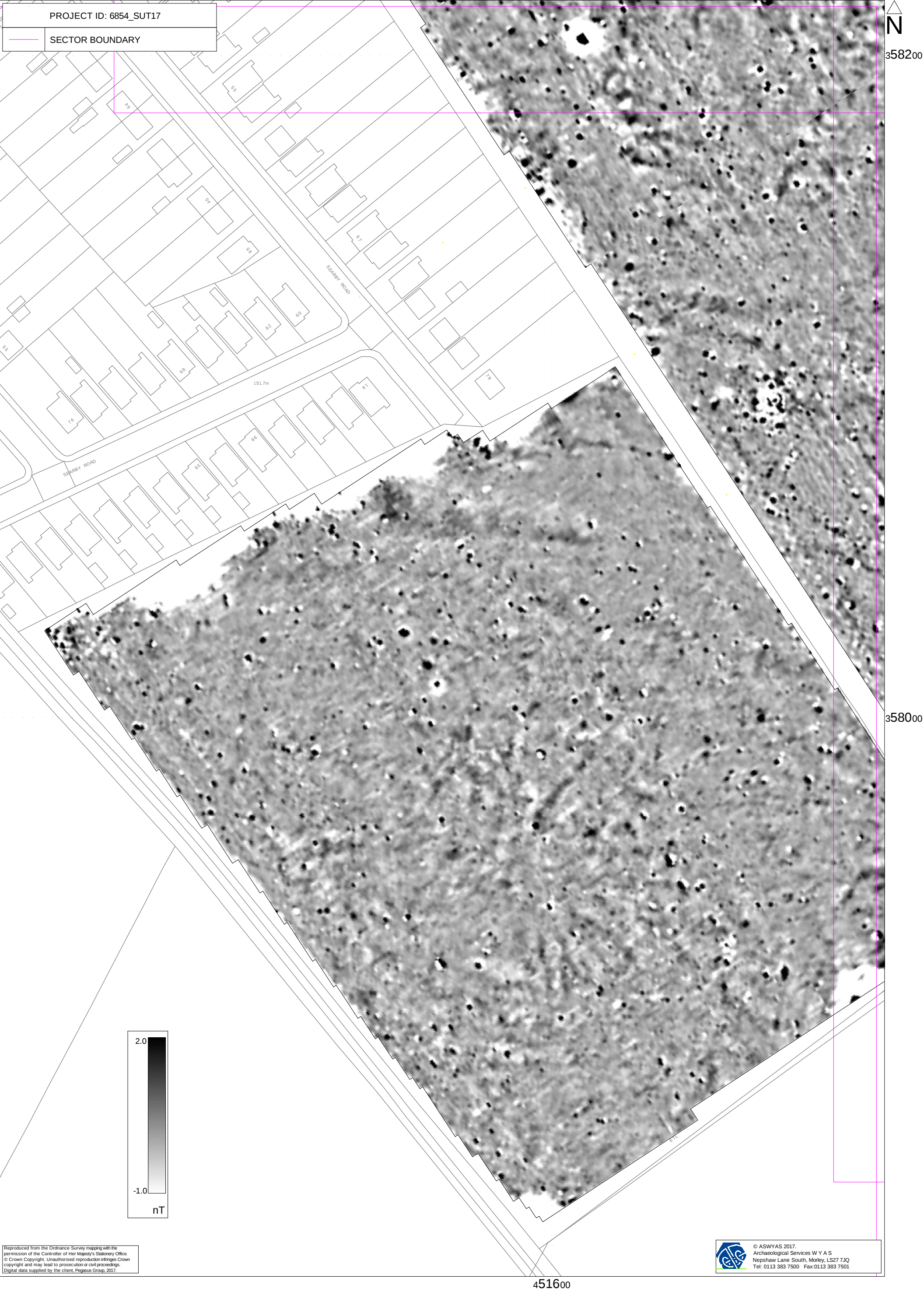
Fig. 13. Processed greyscale magnetometer data; Sector 4 (1:1000 @ A3)
