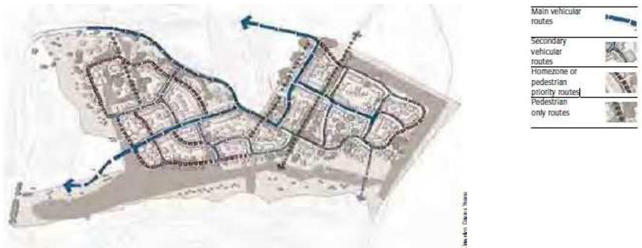
Plan of movement through the site (Llewelyn Davies Yeang) courtesy of Manual for Streets
