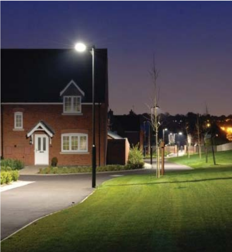
Image showing excessive light spill from a column mounted luminaire – careful luminaire selection and positioning should be used to avoid light trespass such as this.
